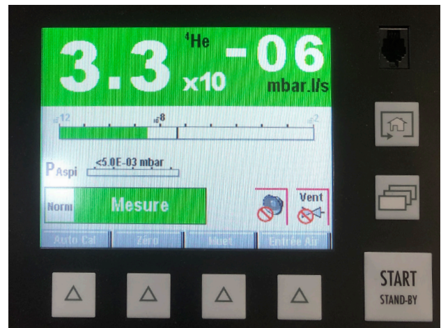
Leak rate < 1 .10-6 mbar.L.s-1 (He)
