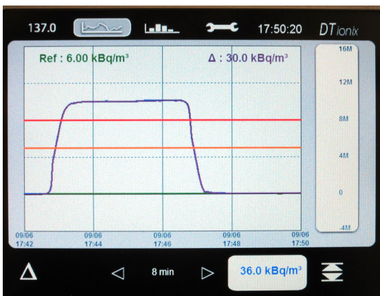
Injection of 10 MBq/m 3 (270 μCi/m 3 ) in a C IONIX 3 - BLC
