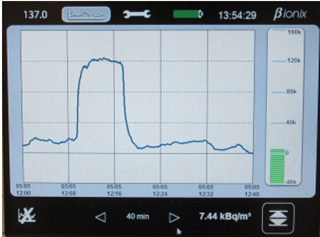
Example of the response at 100 kBq/m 3 (2.7 µCi/m 3 ) B IONIX 3 – MES Volumetric activity measured
