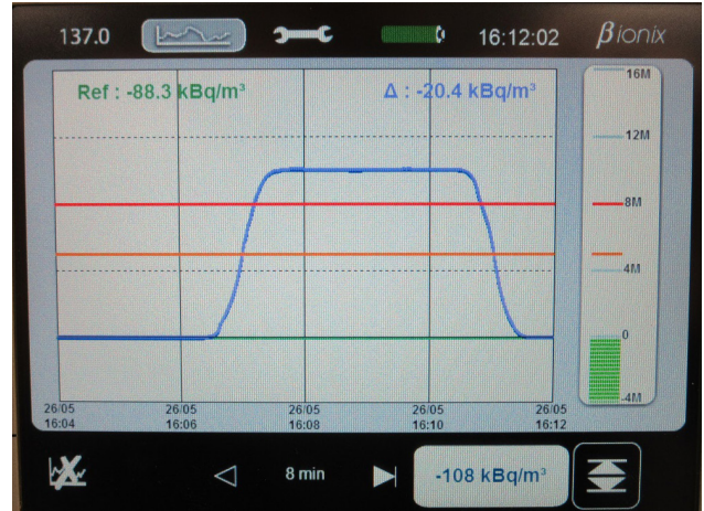
Example of the response at 10 MBq/m 3 (270 µCi/m 3 ) B IONIX 3 – CMP Volumetric activity measured
