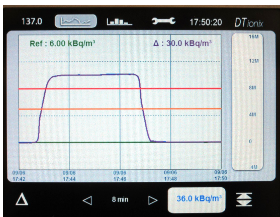
Injection of 10 MBq/m 3 (270 \mu Ci/m 3 ) in a C IONIX 3 - BLC
