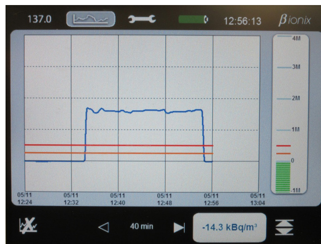
Response to a 1.6 MBq/m 3 (43 µCi/m 3 ) gas injection
