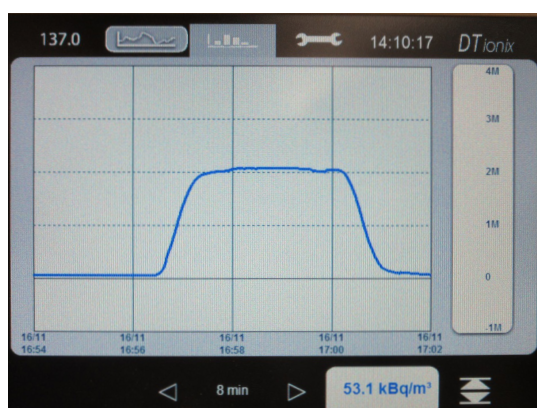
Response to a 2 MBq/m 3 (0.5 mCi/m 3 ) injection
