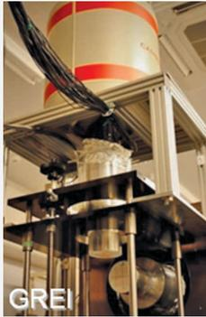
Two Telescopes with each two DSSDs –for the “GREI” project
