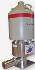
100 pixel detector in a vertical cryostat design
