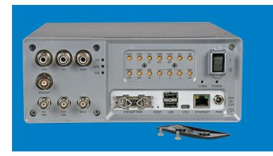
The system's versatility is augmented by its connectivity. For fast local or remote connections, the 10/100/1000 Base-TX Ethernet connection through the RJ-45 port or USB interface are optimal.
